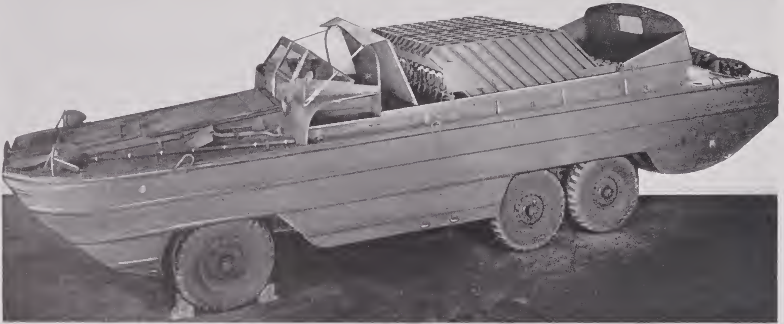
FIGURE 21. Improved Scorpion rocket launcher installed on DUKW.
